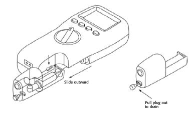
If condensate spills onto the skin or clothing, clean off immediately using fresh water, seek medical advice if problems occur. Ensure plug is replaced before performing combustion tests.
