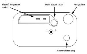
**NOTE:** Take care when inserting the temperature probes as the pins are polarized. Insert with the smaller pin (+) to the right. A view of the sockets is shown below.
