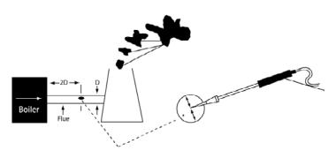
The probe depth stop cone provided with the instrument allows the probe to be used in holes whose diameters range from 1/4 to 4/5 inch (6 mm to 21 mm).
