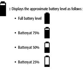
When the display flashes this, it indicates the batteries are at less than 10% of charge and should be replaced, readings may be affected if the analyzer is used with low power batteries.
